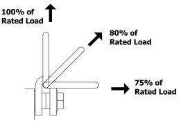
**Important**: The load on each hoist ring is not simply total weight divided by the number of hoist rings. The resultant force can be significantly greater at shallow lift angles and with unevenly distributed loads. See the example below.
